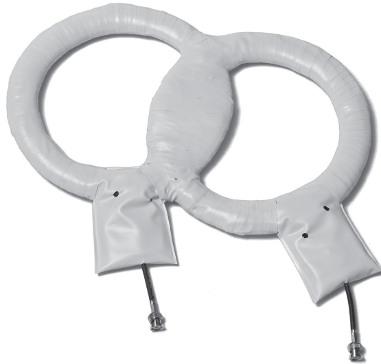
Figure 1. The custom-built quadrature RF transmit/receive surface coil consisting of two 13 cm elements used for our study at 7 T is shown.
