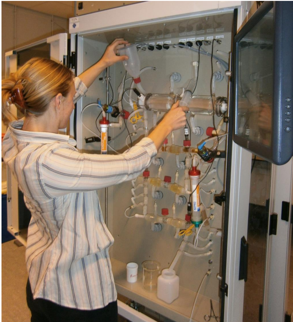
Image 9. Loading the stomach compartment with the tuber meal and removing all excess air in the membrane.
