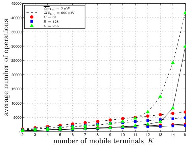
**Fig. 3.9:** Experimental average number of operations as a function of  $K$ , with  $W = 20$  MHz,  $N = 2048$ , and  $R_k^* = R^* = 2$  Mb/s  $\forall k \in \mathcal{K}$  in the case of vacant-carrier assignment model.
