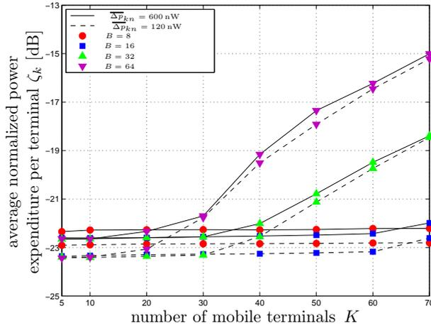
**Fig. 3.4:** Average normalized power expenditure as a function of  $K$ , with  $W = 10$  MHz,  $N = 1024$ , and  $R_k^* = R^* = 200$  kb/s  $\forall k \in \mathcal{K}$  in the case of vacant-carrier assignment model.
