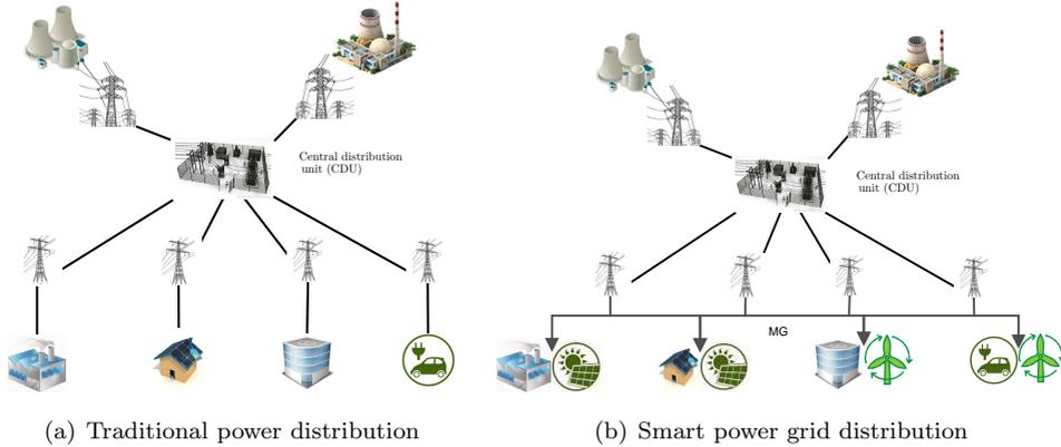
**Fig. 4.1:** *Traditional vs. smart power grid electricity distribution.*
