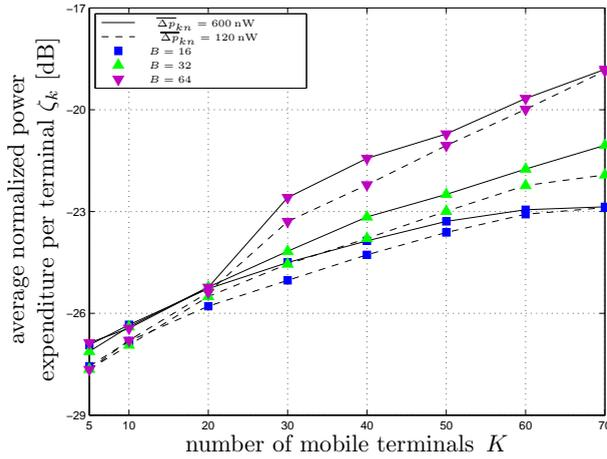
**Fig. 3.6:** Average normalized power expenditure as a function of  $K$ , with  $W = 10$  MHz,  $N = 1024$ , and  $R_k^* = R^* = 200$  kb/s  $\forall k \in \mathcal{K}$  in the case of best-carrier assignment model.
