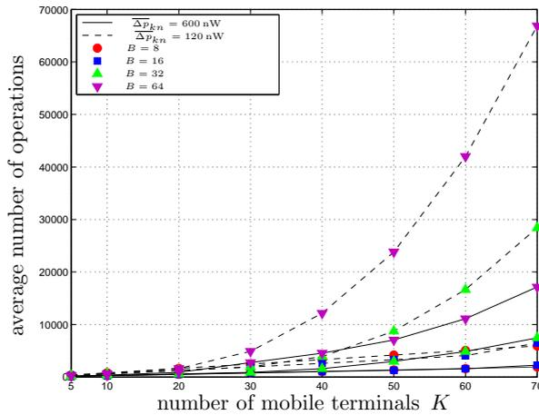
**Fig. 3.5:** Experimental average number of operations as a function of  $K$ , with  $W = 10$  MHz,  $N = 1024$ , and  $R_k^* = R^* = 200$  kb/s  $\forall k \in \mathcal{K}$  in the case of vacant-carrier assignment model.
