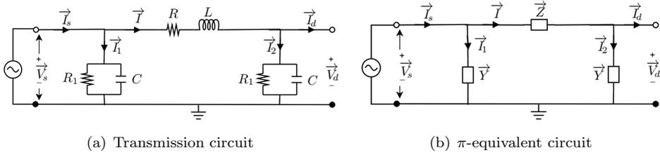
**Fig. 4.2:** Single-phase circuit of a medium-length transmission line.
