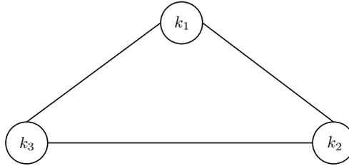
**Fig. 1.1:** The network allocates power among three players according to their will to cooperate with each other. A selfish player receives zero, a pair of cooperative players receive 0.8 mW, and the network supply 1 mW to the grand coalition.
