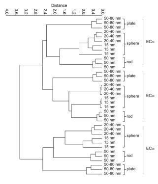
FIGURE 4 | Classifications of four different AgNPs treatments by cluster analysis according to the metabolic characteristics of the microbial communities at the EC20, EC60, and EC90 levels. Two-way ANOSIM, Euclidean-based similarity, n=3, EC level R=0.953,  $\rho=0.0001$ ; shape R=0.876,  $\rho=0.0001$ , respectively.
