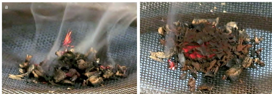
Figure 2. Combustion Experiments with Manganese Dioxide MD4 and Wood Mixtures (a) showing small red flames and volatile emission and (b) the glowing fire combustion phase.
