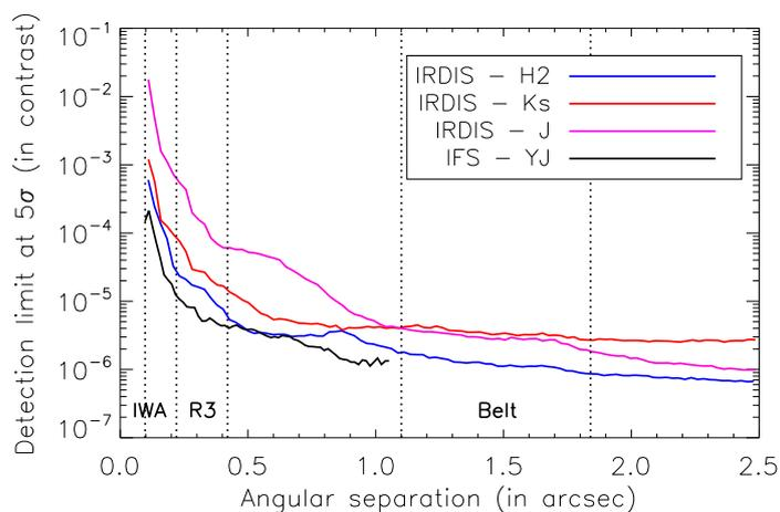
**Fig. D.1.** Detection limit in contrast for YJ, J, H2, and Ks bands with the TLOCI images. The contrast is obtained by an azimuthal standard deviation for each angular separation, corrected by the throughput (SpeCa1, R. Galicher, private communication).
