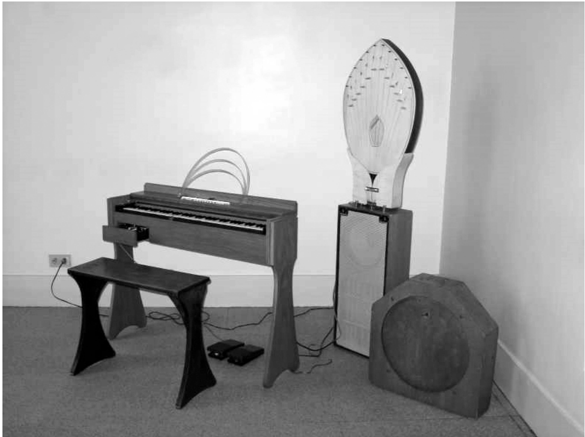
The three different loudspeakers of the ondes Martenot: the palme is placed upon the principal/résonance ., the métalique is at the right.
