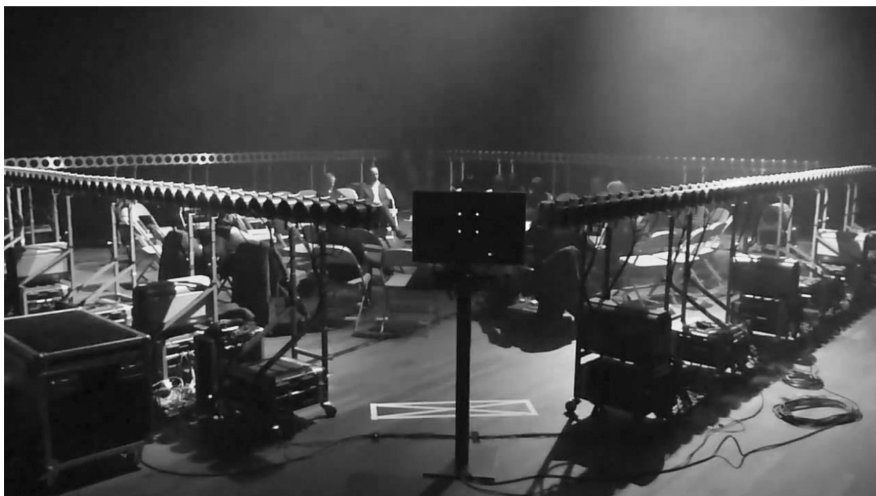
A transportable Wave Field Synthesis system by The Game of Life foundation.
