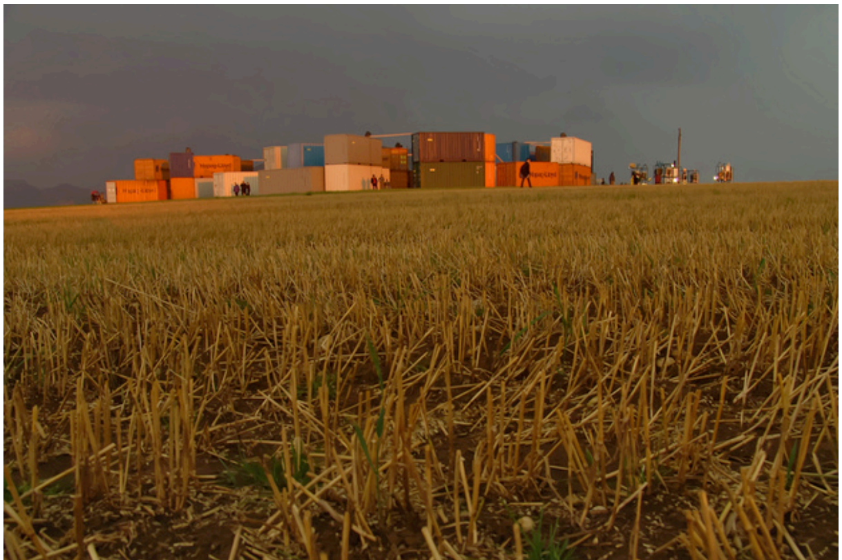
The shipping container village reflected the sounds emitted by the loudspeaker horns, contrary to the hilly landscape.
