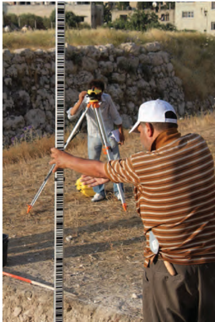
Figure 7.7 Measuring levels inside a square.
