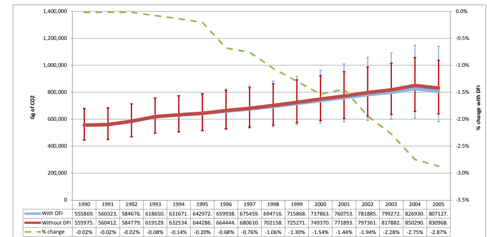
Fig. 6. Calculated scenarios with and without innovation for direct fuel injection (DFI) and percentage change in CO 2 emissions due to the use of DFI.
