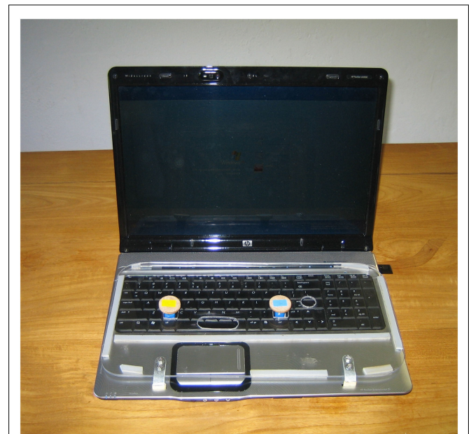
FIGURE 1 | Laptop computer with adjusted response buttons. The computer keyboard was shielded with a perspex plate such that hands and wrists could rest comfortably on the plate, which minimized tremor and prevented unintentional depressing of other keys.
