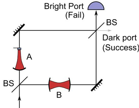
**Figure 1.** The inner interferometer is a Mach–Zehnder interferometer. The upper path contains cavity A which has a weak optomechanical coupling to a resonator. In the absence of optomechanical interaction the interferometer is balanced and all light exits via the bright port. Postselecting only the photons which exit the normally dark port prepares the resonator in its excited state. Cavity B is used to match the spectrum and time delay of cavity A, and has no optomechanical interaction.
