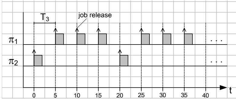
Figure 2.5: Release pattern of jobs of task \tau_3 between processors \pi_1 and \pi_2 , according to the share assignment of \tau_3 in Figure 2.4.
