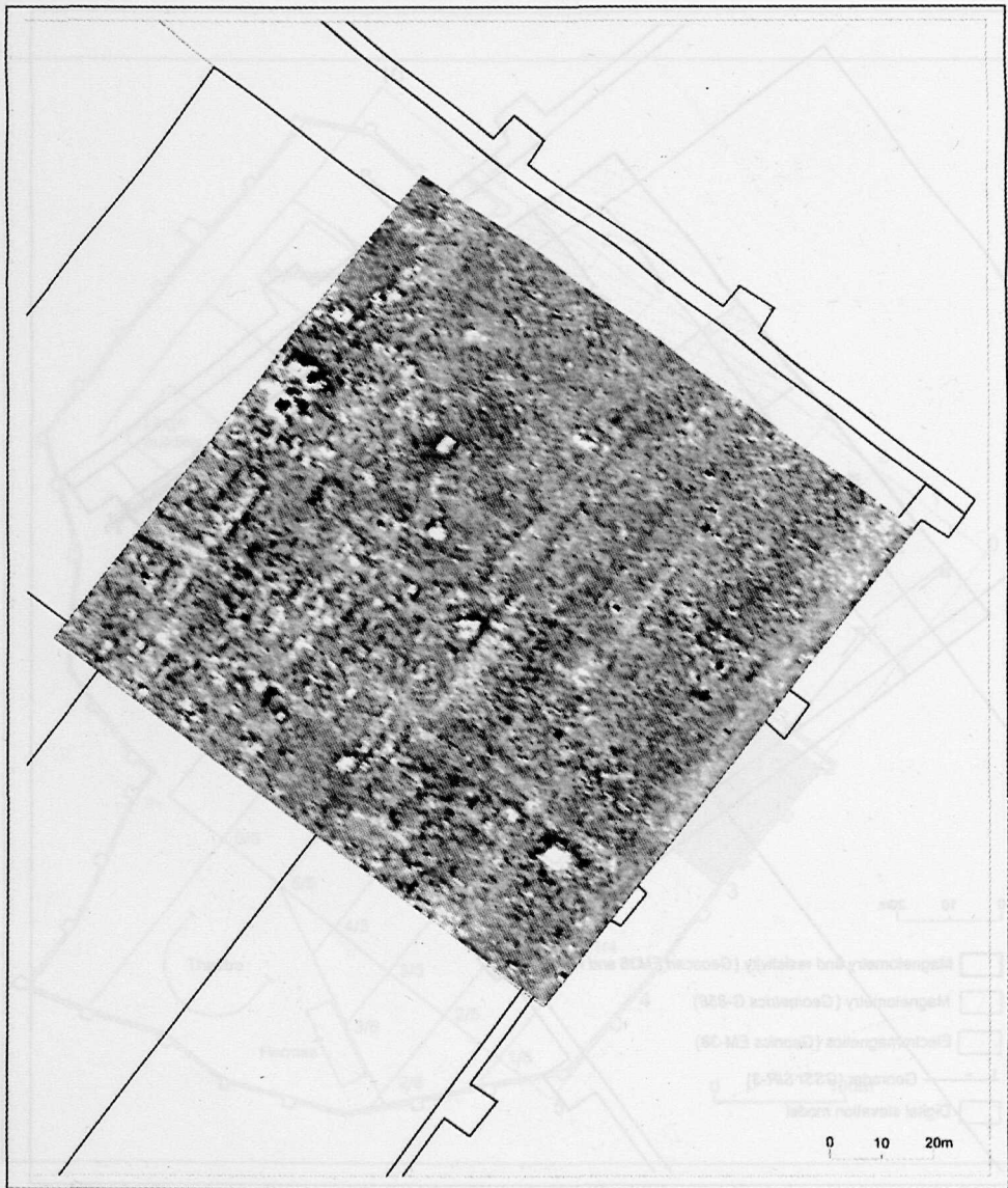
Figure 20. Magnetometry. Vertical gradient of magnetic field (Fluxgate gradiometer Geoscan FM36)
