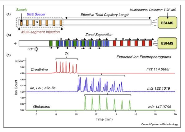
Multi-segment injection in CE-MS. (a) Multiplexed separation based on serial injection of seven discrete sample segments within a single capillary by multi-segment injection CE-MS; (b) ions migrate as a series of zones in free solution before ionization; (c) the procedure enables reliable quantification of polar metabolites and their isomers in different samples as ionization occurs within a short-time interval (≈2–6 min) under steadystate conditions when using ESI-MS.
