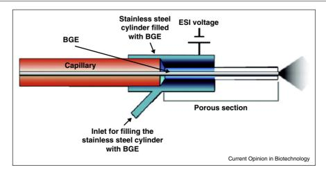
Design of the sheathless porous tip interface. A scheme of the porous tip interface, originally developed by Moini, is depicted. *Source*: Reproduced from [43] with permission.
