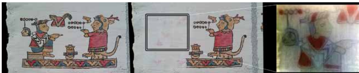
Figure 6.7: Test sample partially covered with new gesso layer and the resultant image from Photothermal tomography (image by Zaman).
