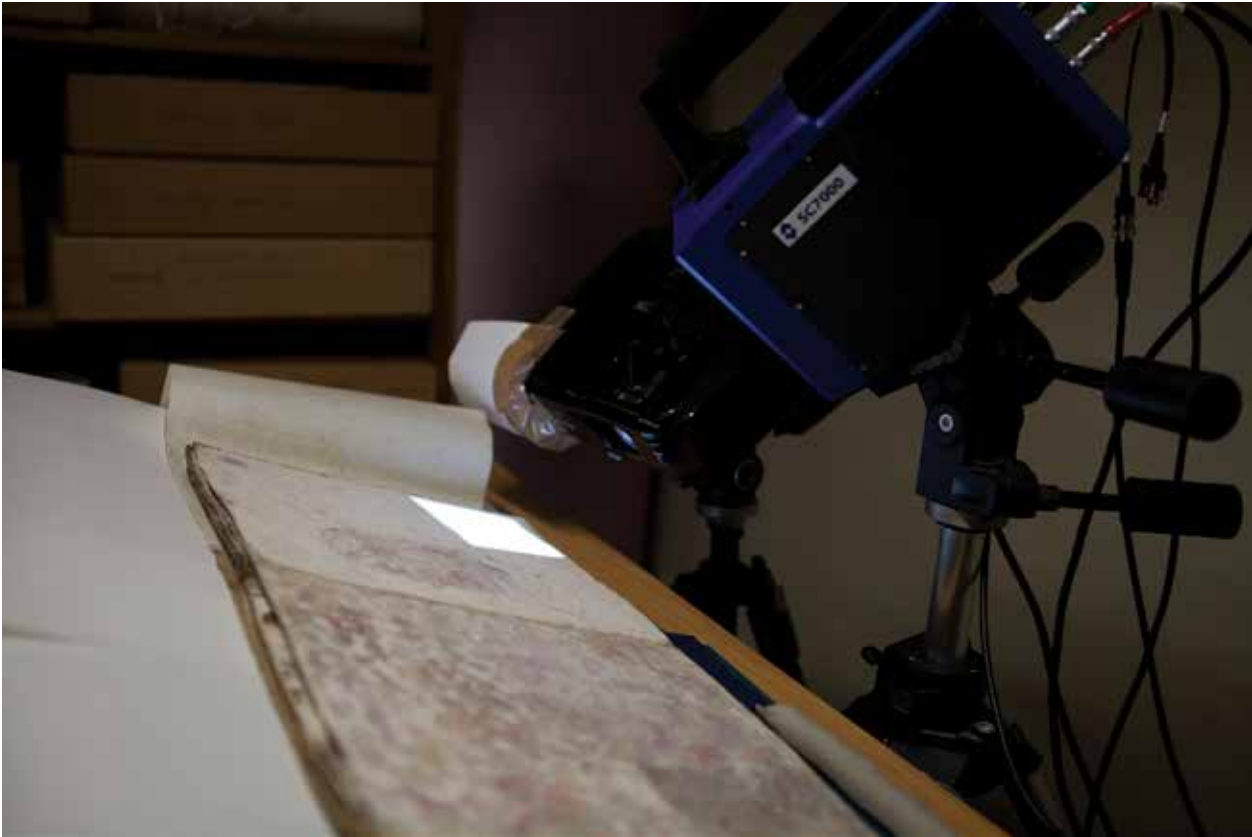
Figure 6.8: Setup of the Photothermal tomography prototype at Bodleian Library during the 2013 investigation of the Añute palimpsest (photo by T. Zaman).
