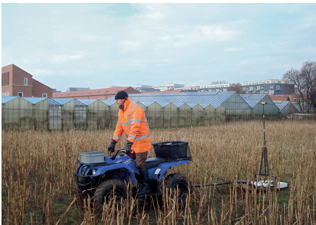
Figure 2 Surveying the site with a groundtracer. Photo: author
