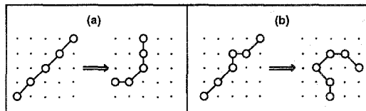
Fig. 3. The saturated string on a 5 \times 5 lattice (a) and the string oversaturated with one hole (b). The characteristic configurations are indicated, as well as configurations which can be reached by a sequence of single-hole hopping processes.
