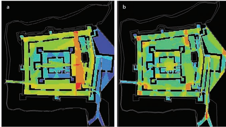
Fig. 4.5 a) Visibility graph of Belvoir: visual integration. b) Visibility graph of Belvoir: visual control.
