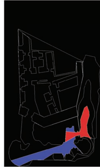
Fig. 5.19 Isovist analysis. The first (red) isovist is taken from the point right in front of the entrance; the second (blue) isovist from the point after entering just beyond the first gate.
