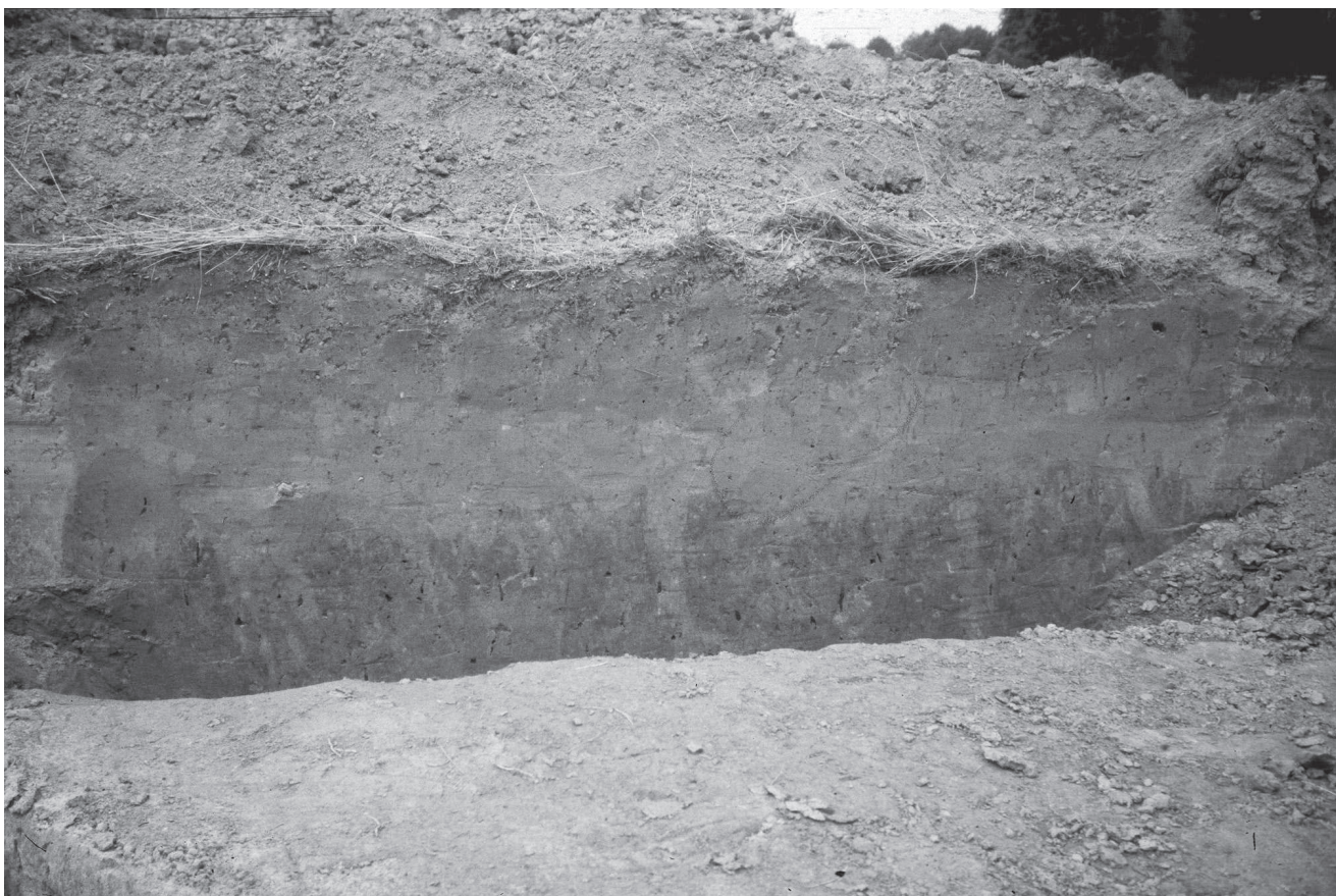
Fig. 3.4 Field photo of a typical soil section, showing the arable, the colluvium and the B_t .
