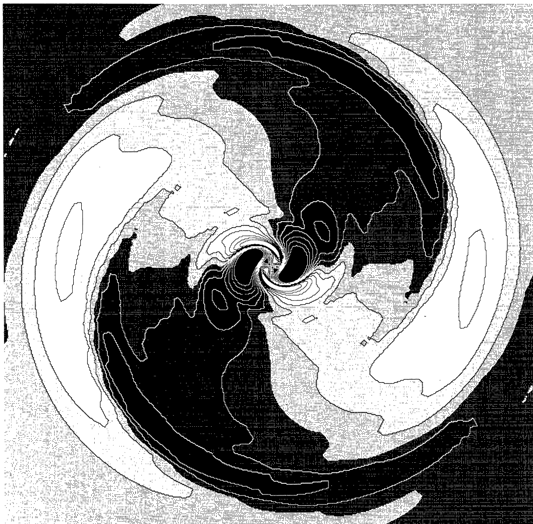
Fig. 9c. The radial velocity scaled to the sound speed, u/c , corresponding with a . Contours are drawn at integer values of the mach number u/c between -6 and 6 . The lighter shades correspond to negative velocities, the darker to the positive
