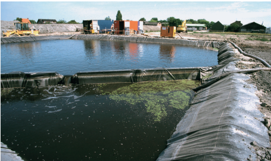
Figure 1.6 Sieving installation in sea container and the artificial decantation basin of the closed-water circulation system.
