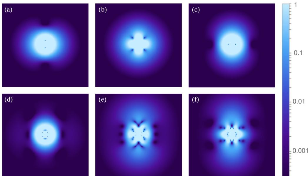
FIG. 3. Energy densities corresponding to  $\mathbf{F}_1$  and  $\mathbf{F}_2$ . (a)–(c) Logarithmic plot of the energy density of the field corresponding to Eq. (12) in the  $xy$ ,  $xz$ , and  $yz$  planes, respectively. (d)–(f) Logarithmic plot of the energy density of the field corresponding to Eq. (13) in the  $xy$ ,  $xz$ , and  $yz$  planes, respectively.
