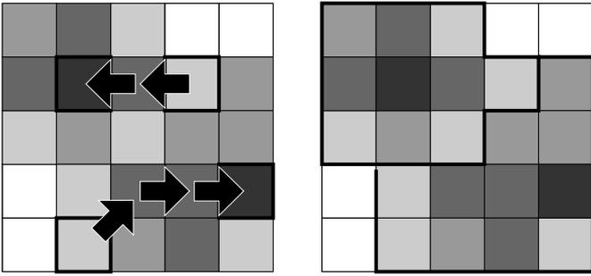
**Fig. 2.** Example in two dimensions illustrating the assignment of pixels to local maxima and the resulting definition of clouds. Starting at the pixels at low intensities (but above the  $1.5\sigma$  level), the algorithm finds the appropriate maximum by moving from brightest neighbour to brightest neighbour. Should a pixel have two equally bright neighbours, the assignment is random. The righthand panel shows the result of the pixel assignment.
