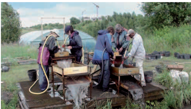
Figure 13 Fractionating the sediment samples using a set of sieves and water (June 2012). (Photo Thijs van Kolfshoten).
